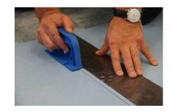
In practice we found it best to detach the half-cut strip with a hooked blade. We do not recommend cutting the underlying edge after embedding the wall covering as this implies the risk of the seam being compressed.
