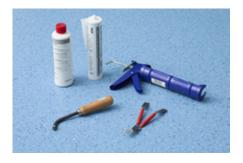
1. Apply nora® liquid wax to seam areas. Leave liquid wax to dry completely!
